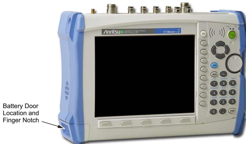
Figure 7-1. Battery Access Door Location and Finger Notch
